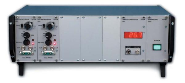
HPD 4.1 is a modular system for measurement of magnetic field by means of Hall probes with high temporal resolution. It consists of a system unit (enclosure, power supply), 1 to 4 Hall probe modules, 1 temperature module and 1 communication module. The system is mounted in a standard 19 inch rack. This driver is primarily designed for magnetic field measurement in fusion research (tokamaks, stellarators), but its application is much broader (industry, R&D).
